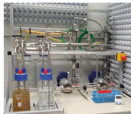
Technical test plant with membrane contactor for nutrient recycling.
