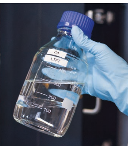
Liquid FT-product with visible aqueous and hydrocarbon phase.
