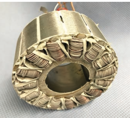
Stator of a synchronous machine in outer rotor construction with polymer-ceramic isolation.
